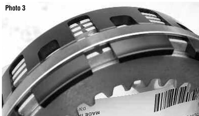
Some vendors, such as Pro-Cutting, hand-grind the friction plate fingers to perfectly fit the tangs of their basket. The resulting gap is very small, yielding a quiet long-lasting clutch.
