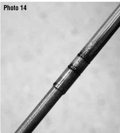
Also check for wear on the clutch pushrod. Failed transmission or pressure plate bearings can cause the pushrod to notch. When this occurs, the pushrod should be replaced. Pushrods will typically have O-rings at one end. On this Ducati pushrod, dual O-rings are used to prevent oil from getting past the left side of the pushrod.
