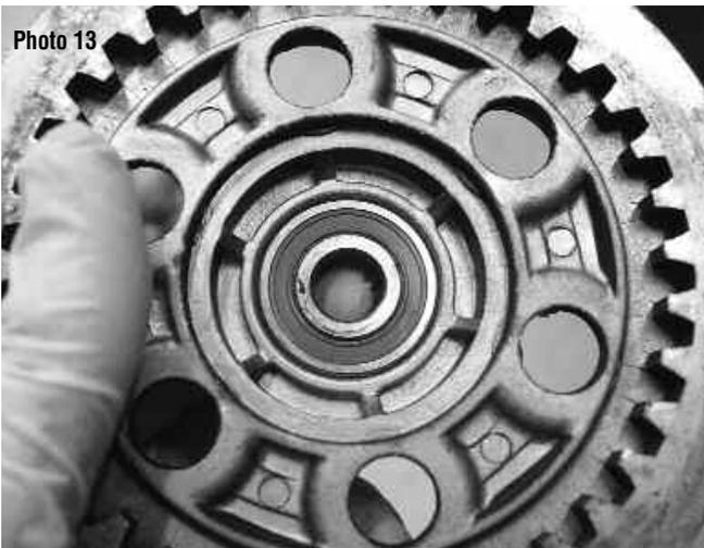
Most owners replace the outer pressure plate for aesthetic reasons. The stock pressure plate, left, doesn't look very good, but will probably last the life of the bike. The only consumable item is the center bearing. Owners should check for wear by placing a finger in the center and spin the bearing to check for stiction.
