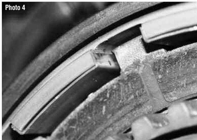
This Barnett clutch basket has steel inserts between the basket tangs to minimize wear. Unfortunately, the gap between the basket tangs and the Barnett clutch pack drive/friction plates isn't optimal, causing premature wear on both the friction plates and the fingers on the basket insert.
