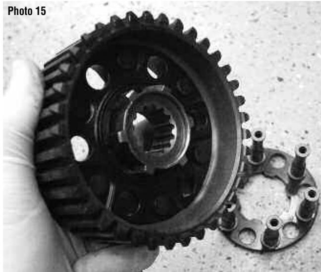
This slipper clutch from Sureflex (available from Motowheels) has the ramps in a two-piece hub—a telltale sign of a slipper clutch. Other slippers will also have a spider-shaped outer pressure ring in lieu of springs and/or ramps with bearings. The ramps are designed to cause the clutch pack to open up during back-torque conditions, thus allowing the clutch to slip. A properly setup slipper clutch slips during back-torque but not during acceleration.
