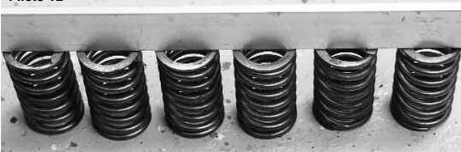
Owners can check for springs that are compressed by laying a straight edge along all six springs. If any of the springs are shorter, replace all six. You can't purchase individual springs.
