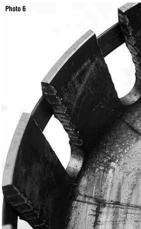
Left: Owners should also check for notching of the basket tangs every 6000 miles. Tangs that are notched more than .75mm should be replaced (my specification). Notches in the basket can cause clutch packs to wear prematurely. New friction plates cannot compensate for the gap caused by worn basket tangs. Worn fingers can only be discerned by removing the pressure plate, several of the friction plates and inspecting the basket.
